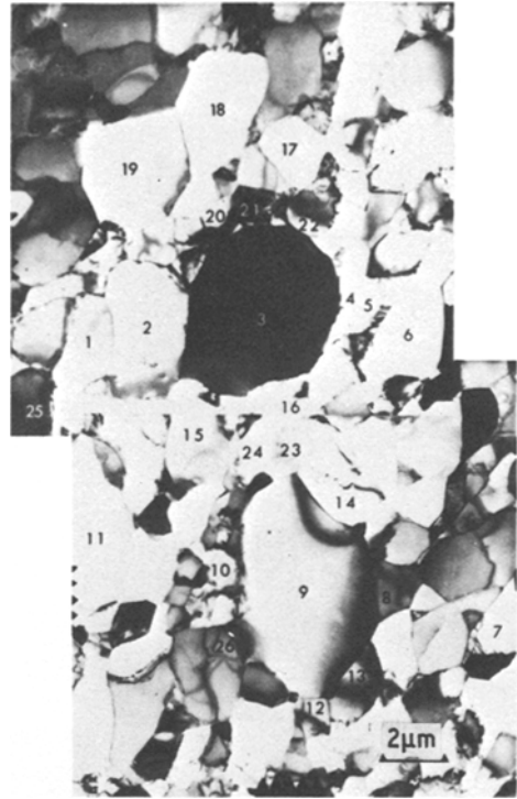
Figure 19 Aluminium compressed 60% and annealed for 2 min at 250° C.
